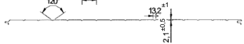
Figure 1: Cross-section of panel type HIPERTEC Wall / SISCOTEK Wall FV 1000
